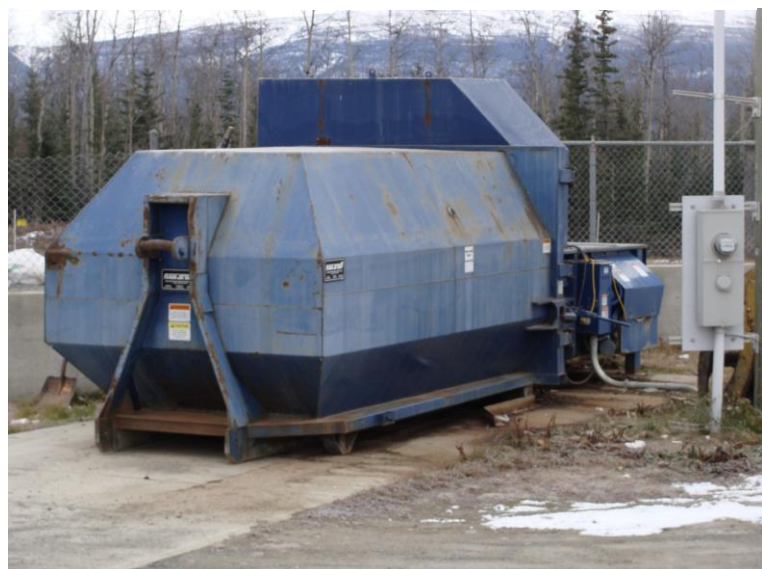
Figure 3. Domestic garbage compactor at Haines Junction landfill
